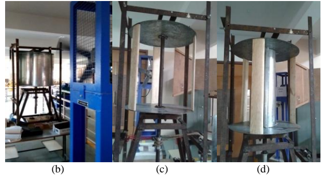
Fig. 4. (a) Schematic diagram of experimental setup, (b) Photograph of Savonius rotor, (c) Photograph of Darrieus rotor, (d) Photograph of hybrid turbine.
