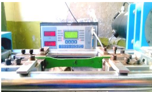
Fig. 3. Photo of Tensometer with FRP and HDPE specimen.
