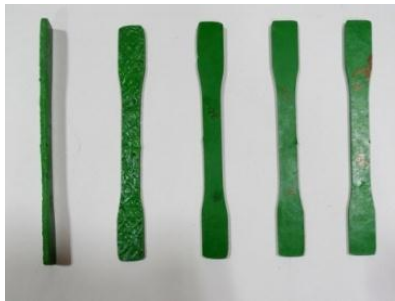
Fig. 2. Photo of specimen obtained after water jet machining.
