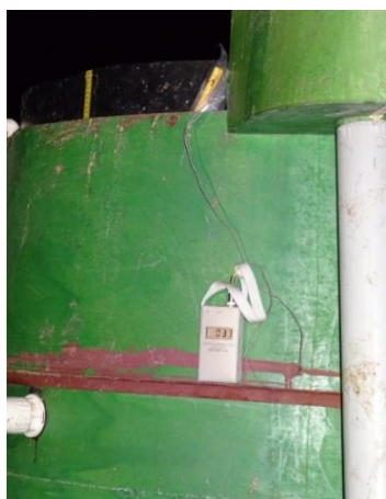
Fig. 14. Photograph of probe thermometer employed to obtain inside temperature of digester.
