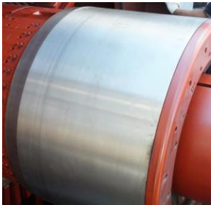
Fig. 6. No marks on retaining ring surface.
