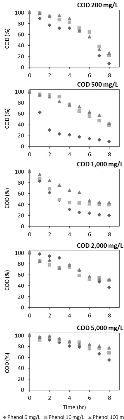
Fig. 2. COD removal by AS with different COD and phenol concentrations.
