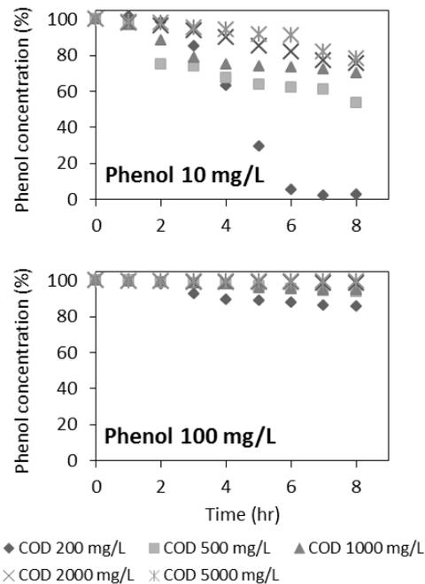
Fig. 3. Phenol removal by activated sludge with different COD and phenol concentrations.
