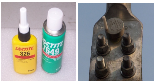
Fig. 3. Temperature sensor installation method
