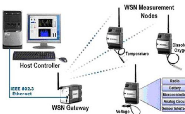
Fig. 1. Temperature monitoring system structure
