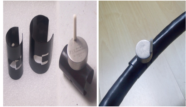
Fig. 4. Temperature sensor installation method
