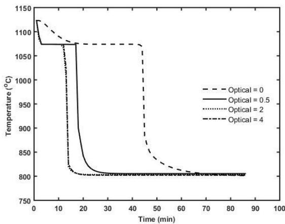
Fig. 4. The effect of optical thickness on the center point temperature.
