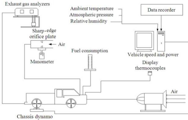
Fig. 1. Schematic of experiment set up.
