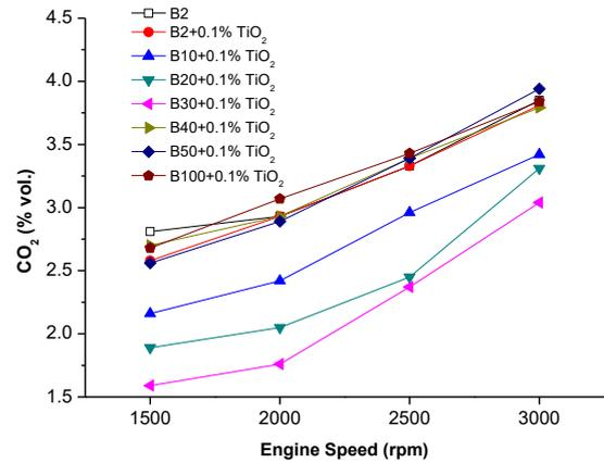
Fig 5. Variation of CO<sub>2</sub> emission for different POB fuels with 0.1%wt nano-TiO<sub>2</sub> additive comparing with B2 standard fuel.
