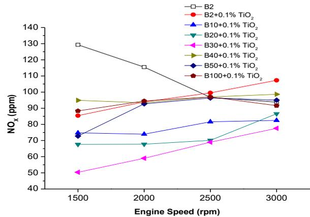
Fig 6. Variation of NO<sub>x</sub> emission for different POB fuels with 0.1%wt nano-TiO<sub>2</sub> additive comparing with B2 standard fuel.
