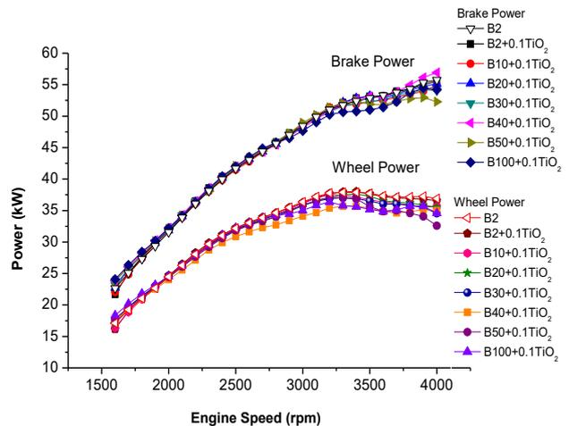
Fig. 2. Power of the engine to consume the different POB fuel blends comparing with B2.
