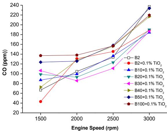
Fig. 4. Variation of CO emission for different POB fuels with mixing 0.1%wt nano-TiO<sub>2</sub> comparing with B2 standard fuel.
