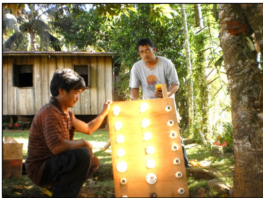
Fig. 7. Measuring the available power at the farthest household being supplied by the MHP.
