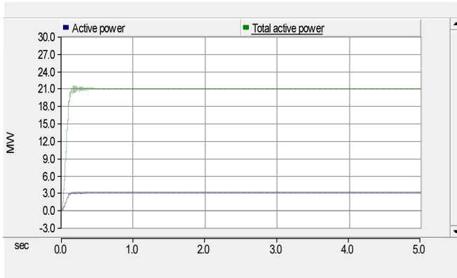
Fig. 8. Active power of 1st hydro generating unit and total active power of Trishuli hydropower plant.
