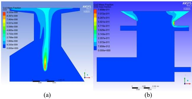
Fig. 6. CO<sub>2</sub> mass fraction: a) PCS-1 and b) proposed cook stove.
