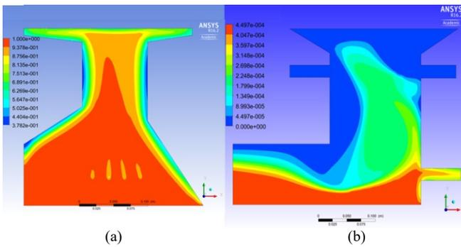
Fig. 7. Mass fraction of soot: a) PCS-1 and b) proposed cook stove.
