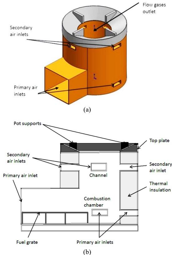
Fig. 2. Proposed cookstove: a) 3D model and b) internal details.
