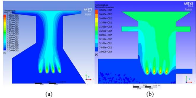
Fig. 4. Temperature contours: (a) PCS-1 and (b) Proposed cookstove.
