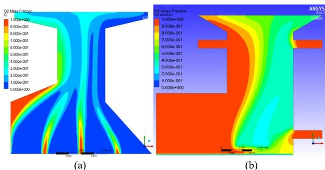
Fig. 9. Oxygen mass fraction: a) PCS-1 b) Proposed cookstove.
