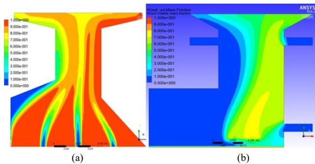
Fig. 8. Wood volatile mass fraction: a) PCS-1 and b) Proposed cookstove.
