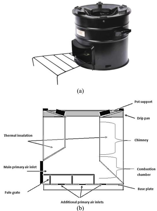
Fig. 1. PCS-1: a) 3D model and b) internal details.
