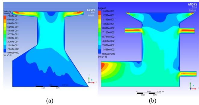
Fig. 5. Velocity fields: (a) PCS-1 and (b) Proposed cookstove.
