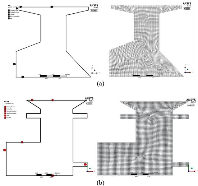
Fig. 3. 2-D computational domain and computational mesh: a) PCS-1 and b) Proposed cookstove.
