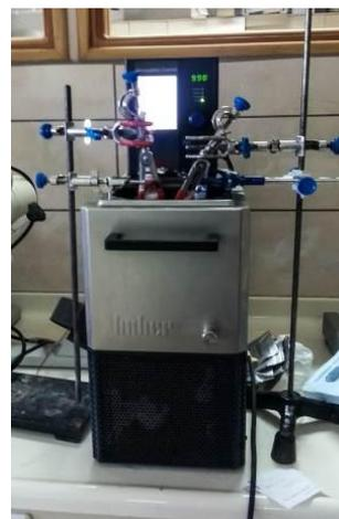
Fig. 2. Experimental setup for heating/cooling curves in waterbath.
