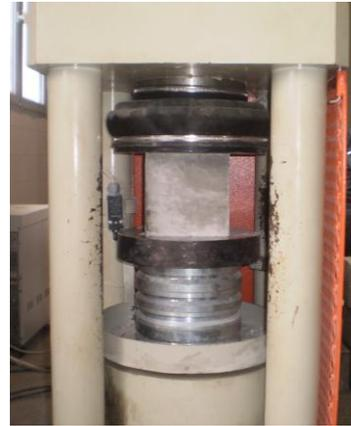
Fig. 3. Universal testing machine for compressive strength test.
