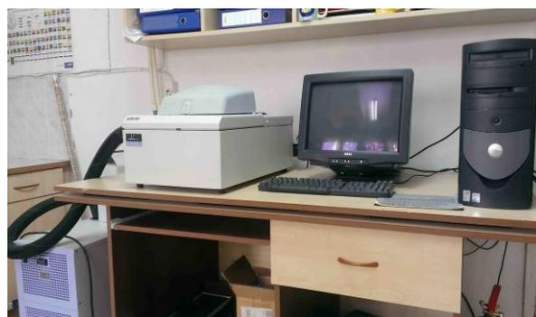
Fig. 1. Differential scanning calorimeter.
