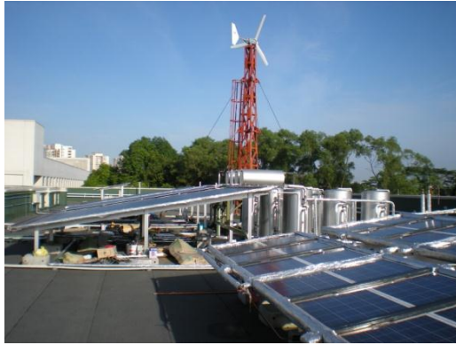
(b). Photo of PV/T test-bed. Fig. 1. Research on the solar PV/T systems in tropical area.
