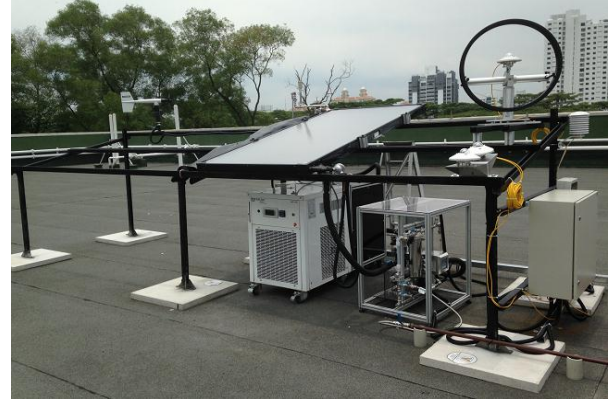
Fig. 4. PV/T testing system setup.
