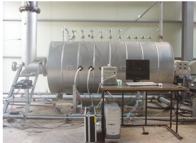
Fig. 4. Experimental setup for liquid burner performance test
