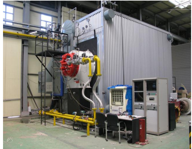
Fig. 3. Experimental setup for gas burner demonstration.
