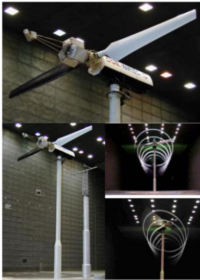
Fig. 2. NASA Ames Research Center full scale aerodynamic complex: NREL Phase VI wind turbine blade [3], [4].
