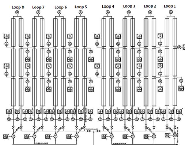
Fig. 2. A schematic of collectors loops of Shiraz solar power plant
