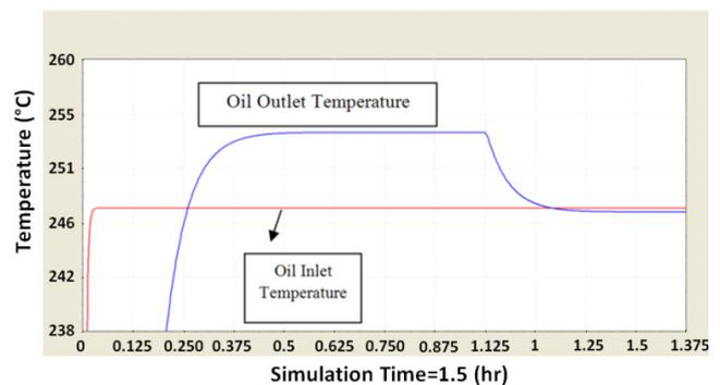
Fig. 4. Variations of inlet/outlet oil temperature of one experimental loop to check response time (modeling)
