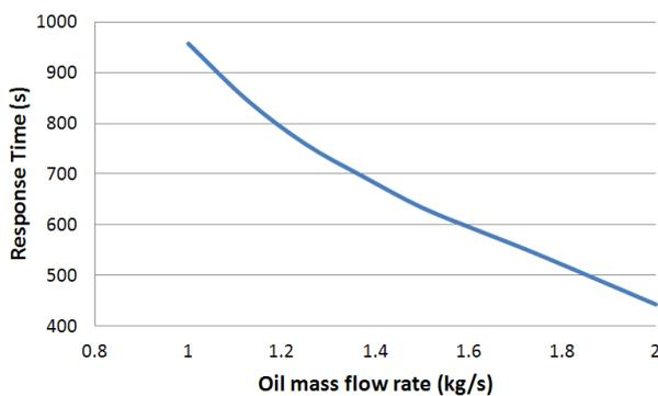
Fig. 3. Responsetime of collector field vs. flow for the first type of modeling
